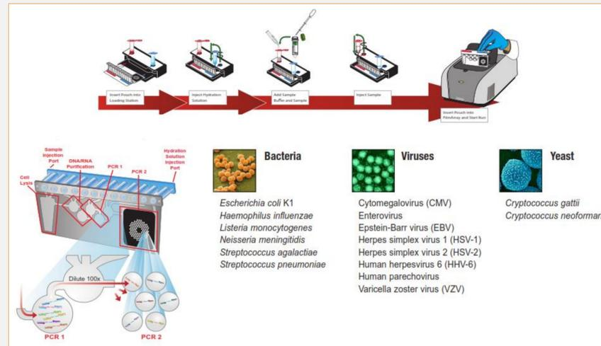
**Figure 2: The FilmArray™ Multiplex PCR System.** The system employs a reagent freeze-dried pouch that stores components necessary for sample preparation, reverse transcription, PCR and detection. The user injects hydration solution and sample combined with sample buffer into the pouch. A nested multiplex PCR is performed in a two-step process and, using endpoint melting curve analysis, a result is generated for each of 16 common pathogens.
